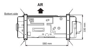
Fix securely with bolts on a solid block. (Use 4 sets of commercially available M10 bolt, nut and washer.)
