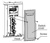
(2) Connect the power supply cable and the connection cable to terminal. Fasten the power supply cable and connection cable with
