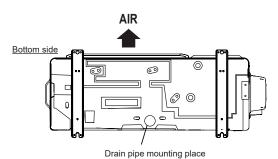
Since the drain water flows out of the outdoor unit during heating operation, install the drain pipe and connect it to a commercial 16 mm hose. (Reverse cycle model only) When installing the drain pipe, plug all the holes other than the drain pipe mounting hole in the bottom of the outdoor unit with putty so there is no water leakage. (Reverse cycle model only)
