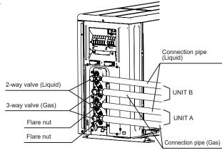
(4) When the flare nut is tightened properly by your hand, use a torque wrench to finally tighten it.
