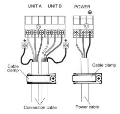
(3) As illustrated, draw out the power cable and the connection cable.
